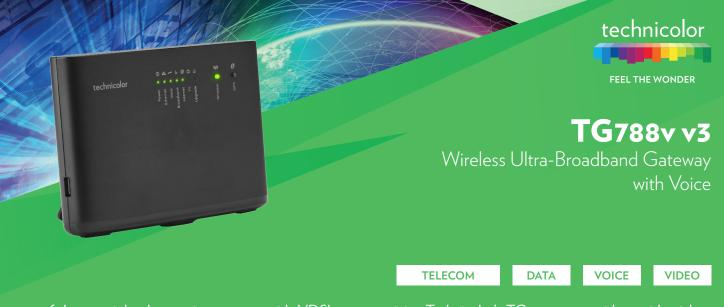
A state-of-the-art triple-play service gateway with VDSL2 connectivity, Technicolor's TG788v v3 provides residential VoIP functions. To get the most from existing infrastructure, the TG788v v3 combines VDSL2 with the latest G.vector and G.inp ("Impulse Noise Protection") technologies. The TG788v v3 features four Fast Ethernet LAN ports and its IEEE 802.11n (2x2) Wi-Fi interface ensures compatibility with existing 2.4 GHz wireless equipment.
