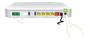
4 The (1) LED turns on. Wait at least two minutes to allow your DGA4130 to complete the startup phase.
