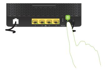
4 The ① LED turns on. Wait at least two minutes to allow your TG788v v3 to complete the startup phase.
