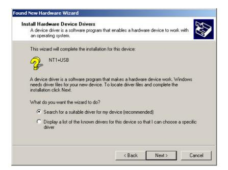
Check CD-ROM drives as an optional search location for suitable drivers. Make sure the NT1+Multi installation CD is inserted in the CD-ROM drive. Then click Next.
