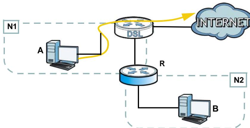
You need to specify a static routing rule on the AMG1302/AMG1202-TSeries to specify **R** as the router in charge of forwarding traffic to **N2**. In this case, the AMG1302/AMG1202-TSeries routes traffic from **A** to **R** and then **R** routes the traffic to **B**.
