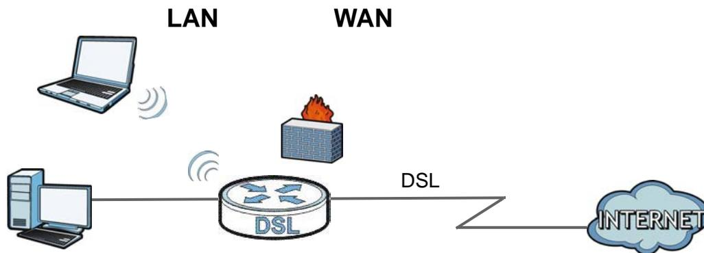
You can also configure firewall and filtering feature on the AMG1302/AMG1202-TSeries for secure Internet access. When the firewall is on, all incoming traffic from the Internet to your network is blocked unless it is initiated from your network. This means that probes from the outside to your network are not allowed, but you can safely browse the Internet and download files.
