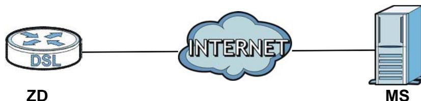
An administrator can use a management server to remotely set up the AMG1302/AMG1202-TSeries, modify settings, perform firmware upgrades as well as monitor and diagnose the AMG1302/AMG1202-TSeries.
