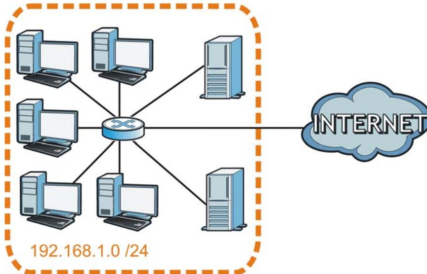
You can “borrow” one of the host ID bits to divide the network 192.168.1.0 into two separate sub-networks. The subnet mask is now 25 bits (255.255.255.128 or /25).
