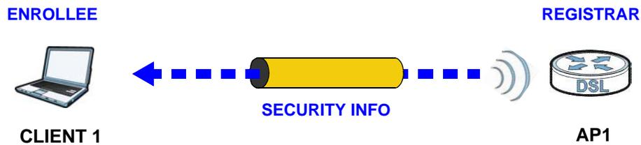
In step 2, you add another wireless client to the network. You know that **Client 1** supports registrar mode, but it is better to use **AP1** for the WPS handshake with the new client since you must connect to the access point anyway in order to use the network. In this case, **AP1** must be the registrar, since it is configured (it already has security information for the network). **AP1** supplies the existing security information to **Client 2**.
