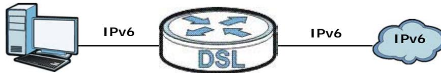
In the **Network Setting > Broadband** screen's **IPv6 Address** configuration section, select **Obtain an IP Address Automatically**. In the **DHCP IPv6** field select **DHCP** to obtain an IPv6 address from a DHCPv6 server. In the **DHCP PD** field select **Enable** to have the AMG1302/AMG1202-TSeries pass the WAN prefix to LAN hosts. The LAN hosts can then use the prefix to generate their IPv6 addresses.
