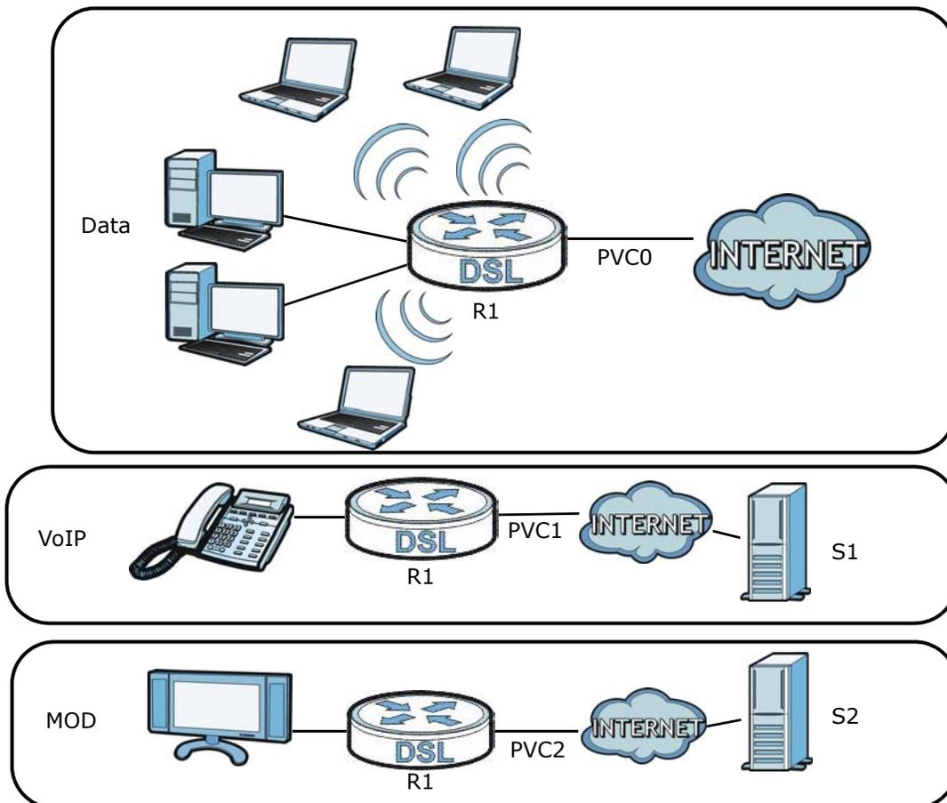
If a WAN PVC is bound to an ethernet port, traffic from the ethernet port will only be forwarded through the specified WAN PVC and vice versa. If a port is not in a port binding group, traffic to and from the port will be forwarded according to the routing table. See the tutorial section ([Section on page 37](#)) for more details on configuring port binding for multiple WAN connections.
