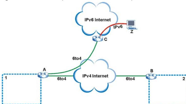
In a 6to4 tunnel, 6to4 routers (**A** and **B** in the example network) forward these packets between IPv6 networks (**1** and **2**) over the IPv4 Internet. A 6to4 relay router (**C**) connects to both an IPv6
