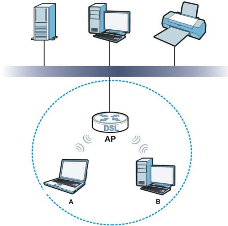
The wireless network is the part in the blue circle. In this wireless network, devices **A** and **B** use the access point (**AP**) to interact with the other devices (such as the printer) or with the Internet. Your AMG1302/AMG1202-TSeries is the AP.
