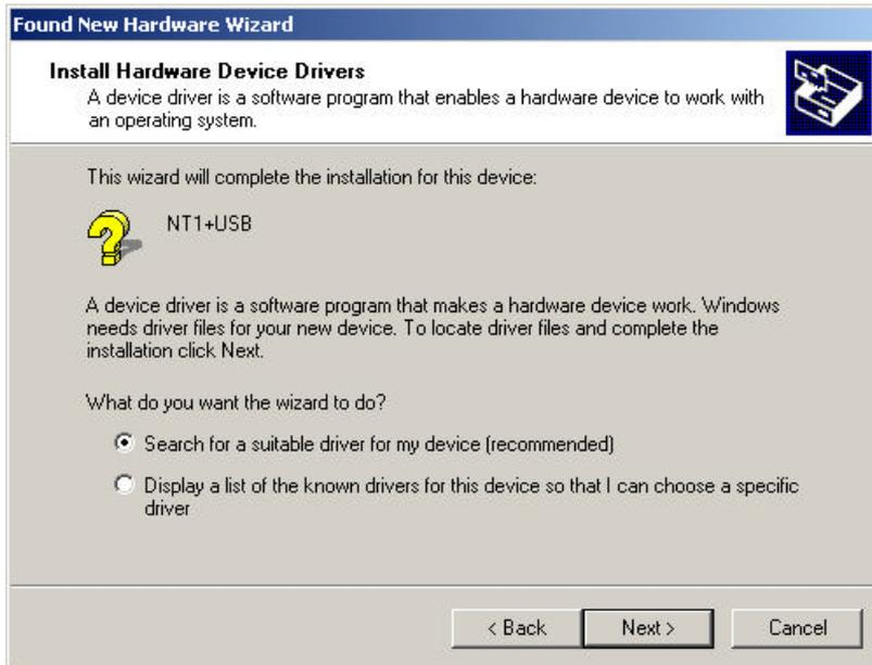
Check CD-ROM drives as an optional search location for suitable drivers. Make sure the NT1+Multi installation CD is inserted in the CD-ROM drive. Then click Next.
